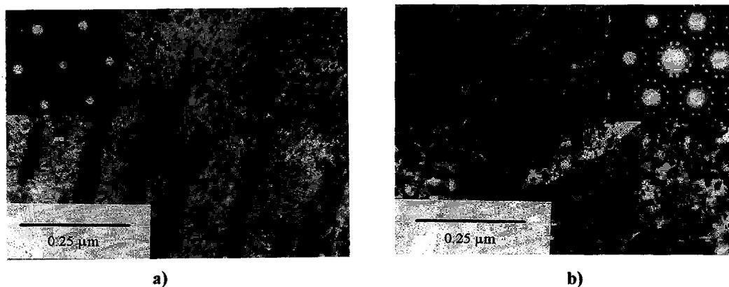
**Figure 4:** Structure of the Ni51.0at.%-Ti alloy deformed by 5% and then aged at 400°C/1h (diffraction patterns in the corners show extra spot from the R phase (a) and  $\text{Ni}_4\text{Ti}_3$  precipitates (b))
