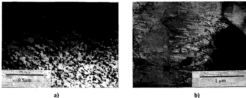
**Figure 3:** Structure of the Ni50.6at.%-Ti alloy deformed by 10% and aged at 400°C (a) and 500°C (b)
