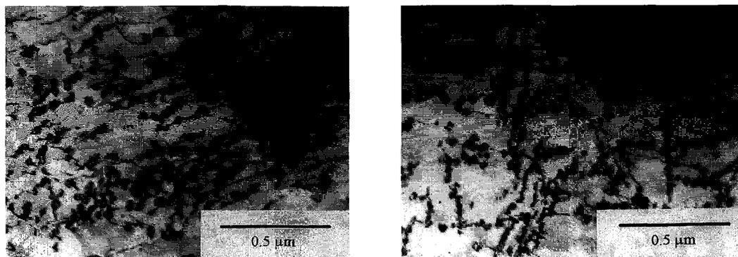
Figure 1: Structure of the Ni50.6at.%-Ti alloy deformed by 5% and aged at 400°C/1h
