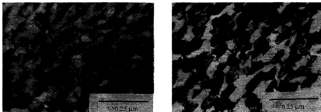
Figure 6: The structure of the Ni51.0%-Ti alloy deformed by 5% and aged at 500°C/1h
