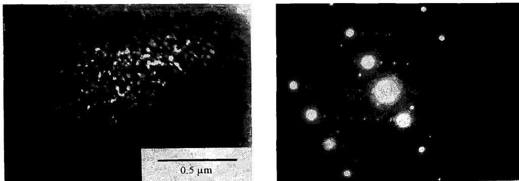
Figure 2: Dark-field image of  $\text{Ni}_4\text{Ti}_3$  particles and the corresponding diffraction pattern in [233] orientation of the Ni50.6%-Ti alloy deformed by 5% and aged at 400°C/1h
